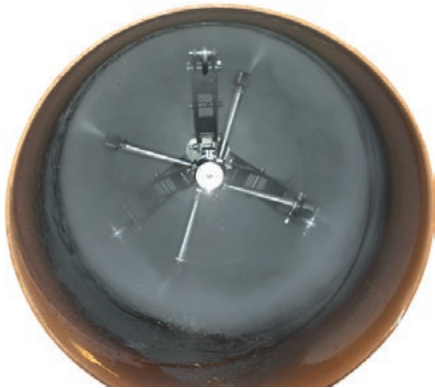
Thorough Water Jetting Unit for cleaning of the pipe
